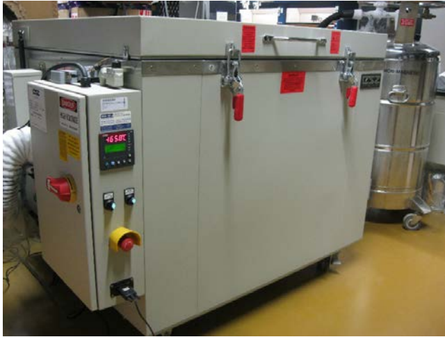
Concrete samples in LN 2 -cooled temperature chamber
