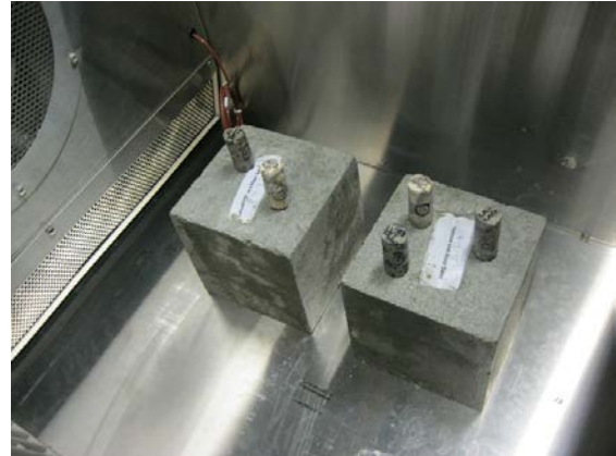
Concrete samples in LN 2 -cooled temperature chamber
